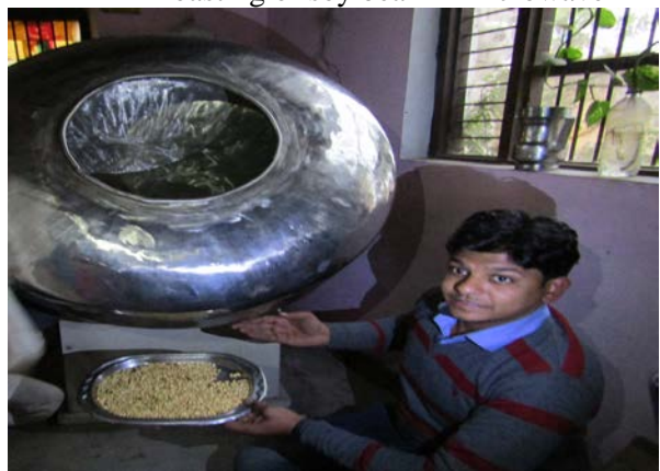
Hands on training about mixing of spices with roasted soynuts in spice coating machine
