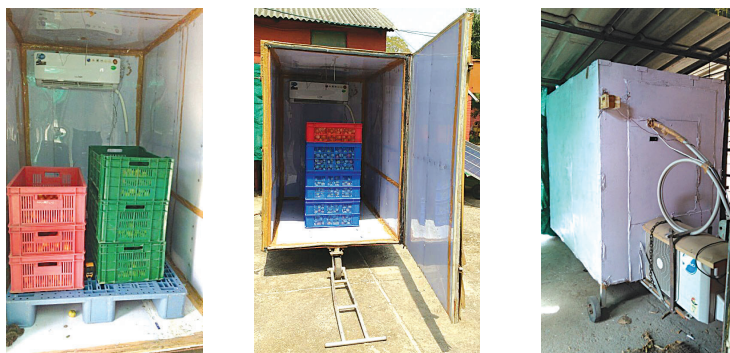
Solar powered movable cold storage structure with 0.8 ton AC connected and stored tomato
