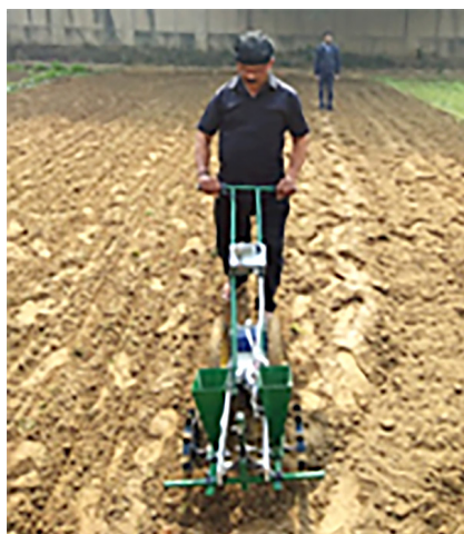
Battery assisted spinach-cum-coriander seeder
