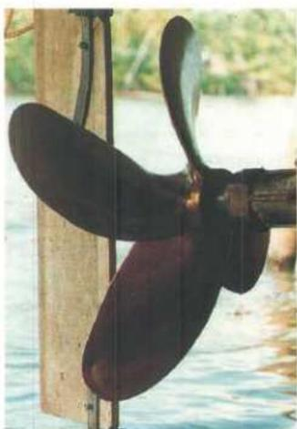
The redesigned curvatures of the blades have lent efficiency to the 4-blade propellers fitted on the existing medium-sized trawlers of 100 HP range operating off Kerala coast. While the fuel efficiency is 30% for the corresponding speed and pull, the load on the engine considerably less, CIFT, Cochin
