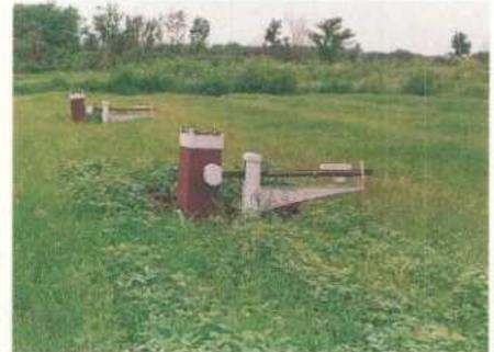
A Lysimeter has been developed to measure the specific requirement of water at various stages of crop growth
