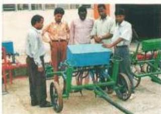
Animal-drawn multipurpose tool carrier may be fitted with tillage, sowing or interculture equipment
