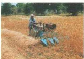
Self-propelled vertical conveyor reaper-harvester
