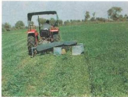
IGFRI ROTARY DISC MOWER has been designed for harvesting berseem and the oat crops. Its capacity is 0.22 hectare per hour and efficiency, 62%
