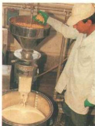
Wet-grinding of soybean for tofu-making, CIAE, Bhopal. The technology is being widely used in the country
