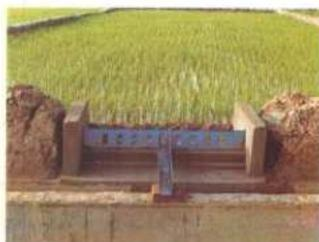
Excess rainfall in rice fields is measured by this device developed by the Water Technology Centre for Eastern Region, Bhubaneswar, Orissa
