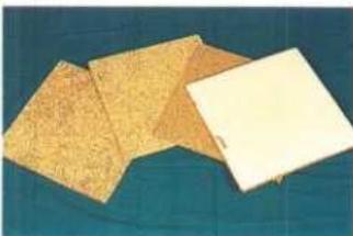
Particle boards manufactured from jute-and-cotton residues
