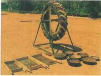
IGFRI TYRE-TYPE SEED PELLETING MACHINE can produce 20-25 kg of seed pellets in an hour
