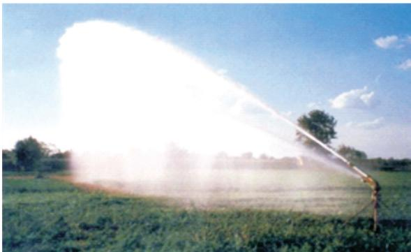
**Fig. 5.9: Rain gun installed in field**
