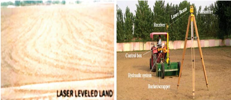
**Fig. 1.8: Laser leveller in operation**
