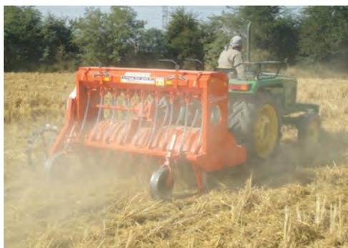
*Fig. 8. A 'Happy Seeder' for direct drilling of seeds in the presence of surface residues (Courtesy: CSISA, CIMMYT-IRRI, New Delhi)*
